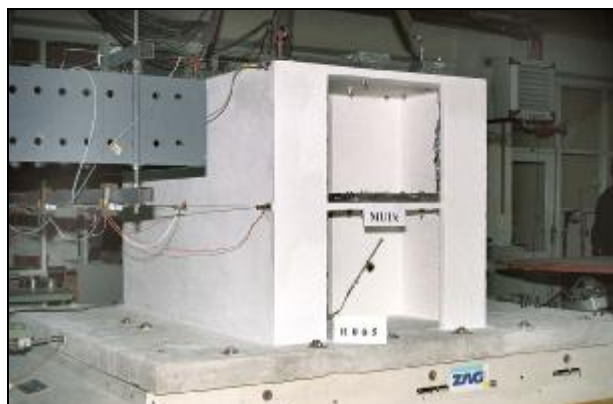
Slika 2. Tipičan model vrstne kuće na početku ispitivanja Figure 2. Typical model of a peak house at the start of testing
