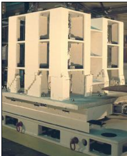
Slika 5. Model stambene kuće M2-2 u fazi rušenja Figure 5. Model of a residential house M2-2 in collapsing phase
