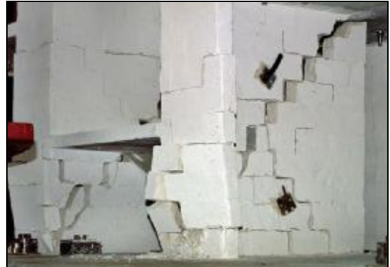
Slika 8. Oštećenja 4. stepena pre rušenja (Model M2-2, \Phi = 1,77\% ) Figure 8. Grade 4 damages prior to collapse (Model M2-2, \Phi = 1.77\% )
